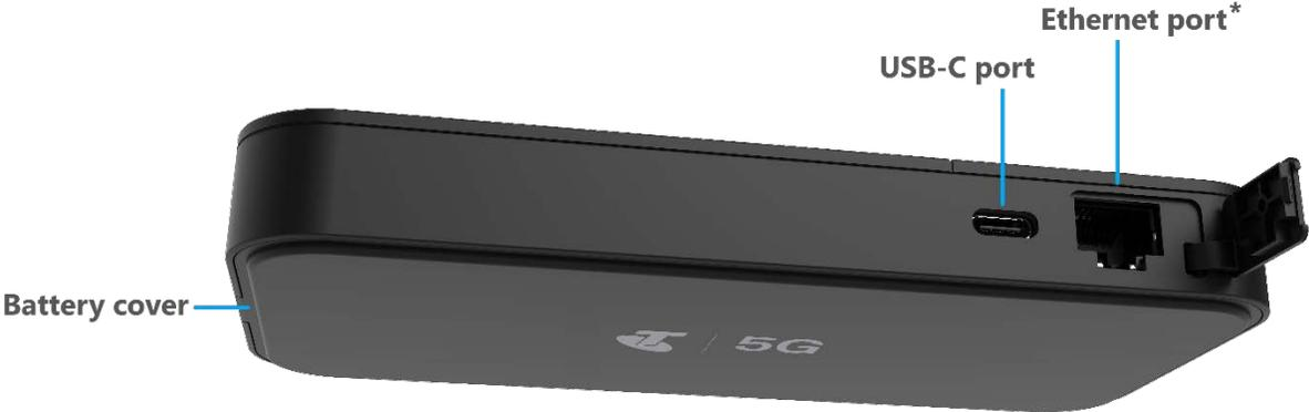
\*To reduce power consumption, the ethernet port is deactivated by default. You can activate it from the touchscreen (Menu > Settings > Enable Ethernet Port), or from the Admin web UI (Settings > Preferences > Enable Ethernet Port).
